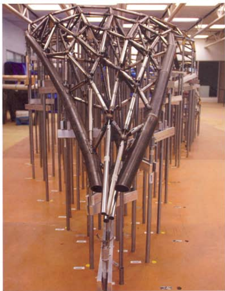
ABOVE A 1:6 MOCK-UP OF THE STEEL STRUCTURE INCLUDING ALL CONNECTIONS FOR ONE WING OF THE BAHÁ'Í TEMPLE HAS BEEN FABRICATED AT SOHEIL MOSUN LIMITED IN TORONTO. SHOWN ARE COMPARATIVE IMAGES OF THE COMPLETED PHYSICAL MOCK-UP AND THE CATIA VIRTUAL MOCK-UP.
