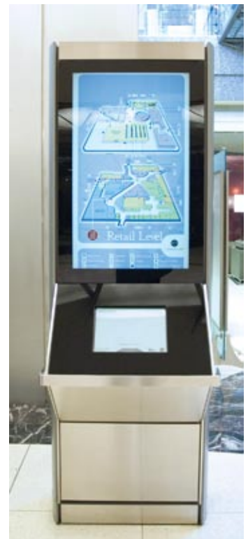
Computerized touch-screen building directory
